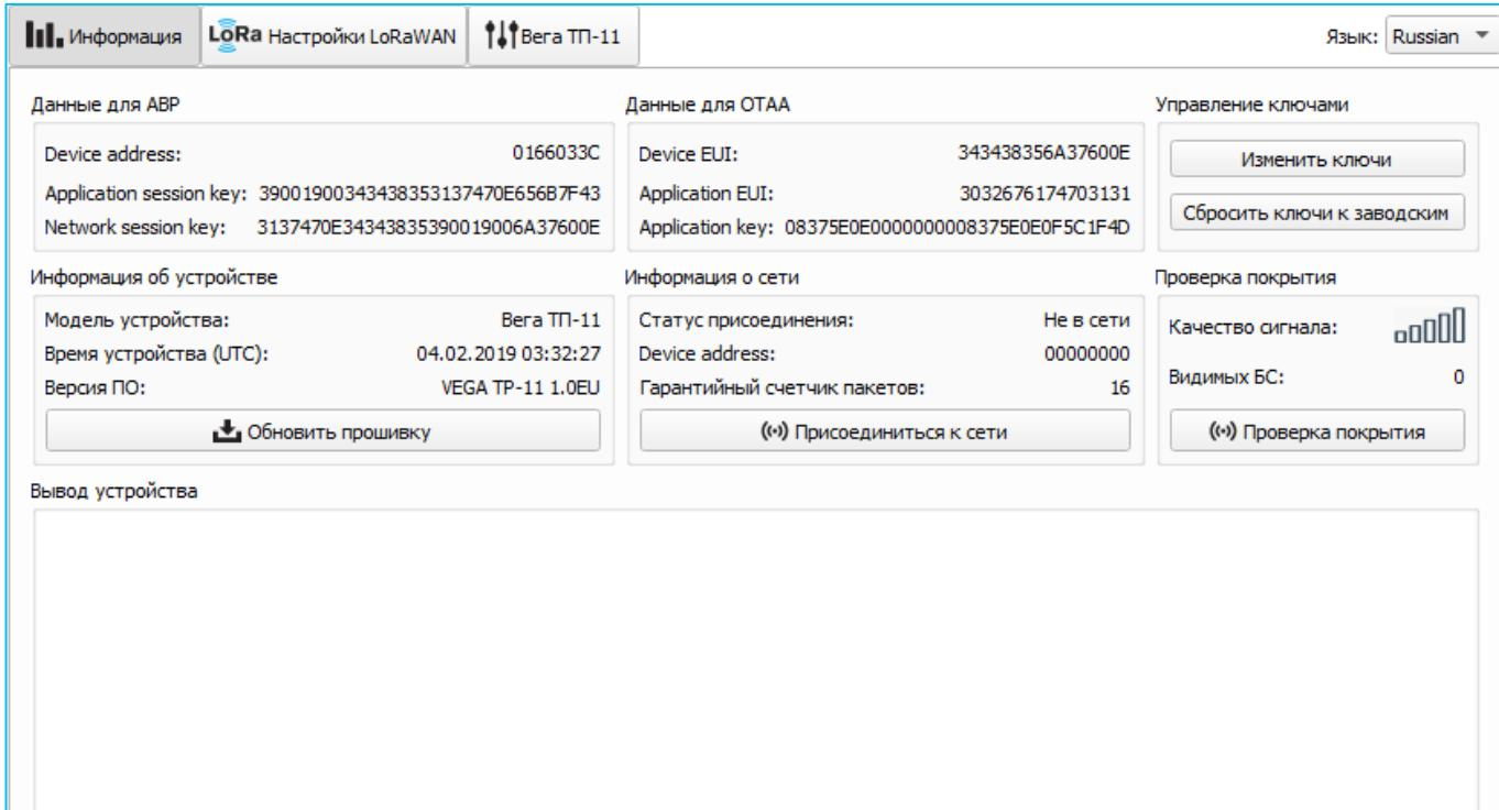
The screenshot shows the 'Information' tab of the VEGA TP-11 configuration interface. It includes sections for ABP and OTAA parameters, key management, device information, network status, and coverage testing.
